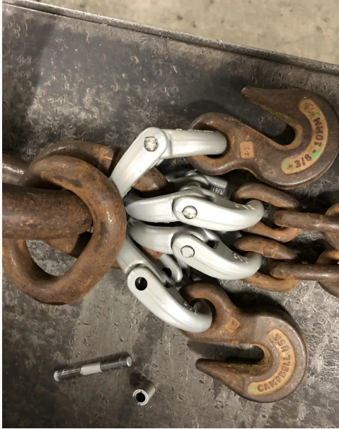
Chain sling stripped down for re-build and proof test.
